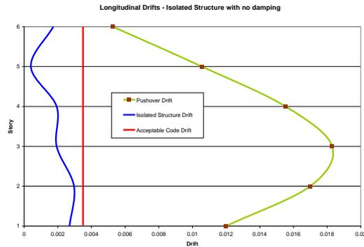
Fig 8 - Comparative story drifts for base isolated structure
