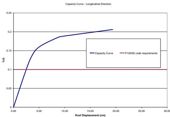
Fig 7 a) Capacity curve of fixed base model
